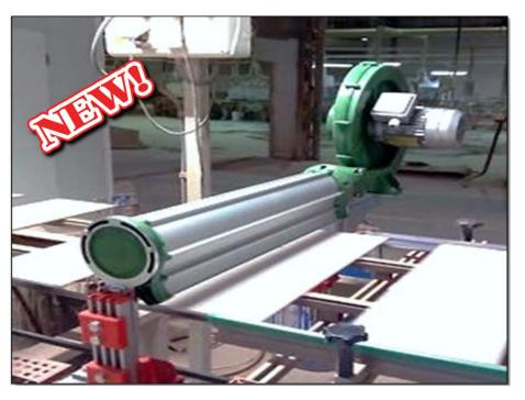
The Transversal Diffuser has been designed to clean/cool/dry large sizes tiles. Optimized for the use with GreenBlow, it allows to obtain an "airblade"up to 3200 mm. High versatility of use is provided by the ease of assembly and by the wide diffuser rotation. Two configurations are realized: with direct inlet and with 90 ° inlet.
